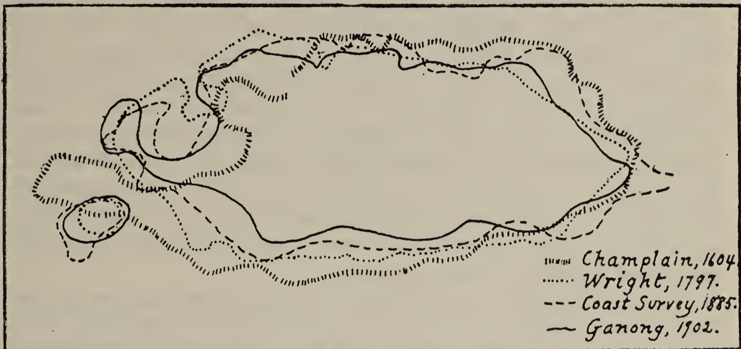
FIG. 8.—The four principal maps of Dochet Island reduced to the same scale and superposed.
